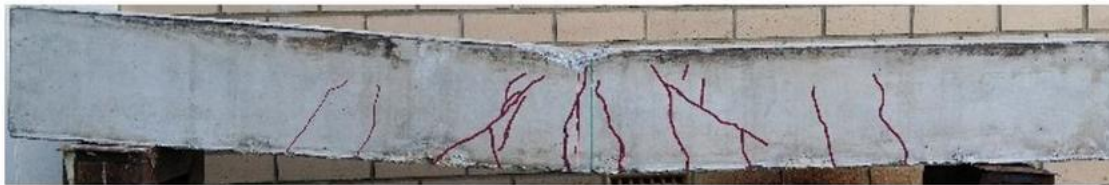
Failure under impact load
