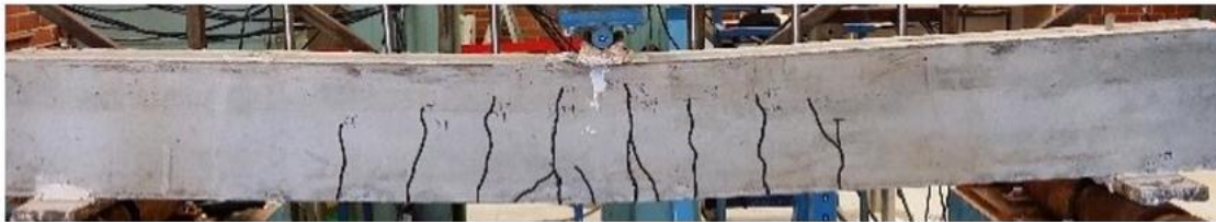
Failure under static load
